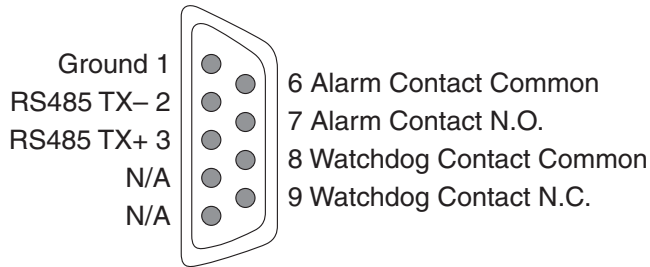
Alarm & PTZ Wiring Diagram
