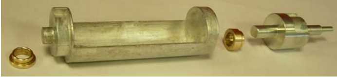
L to R: Rear Bushing, Casting, Front Bushing, Spindle
