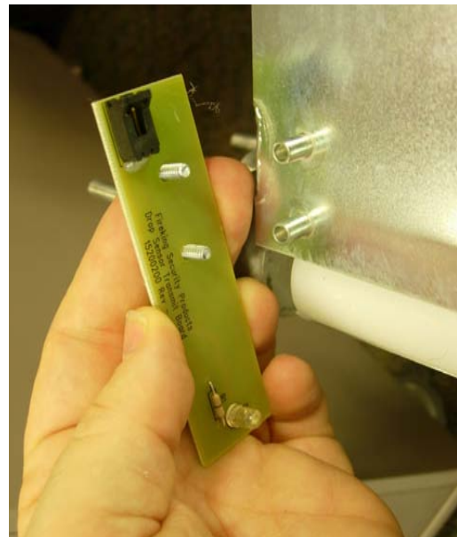
Disconnect Drop Sensor Boards (ex. shown left) or Remove Drop Sensor Boards (ex. shown right)
